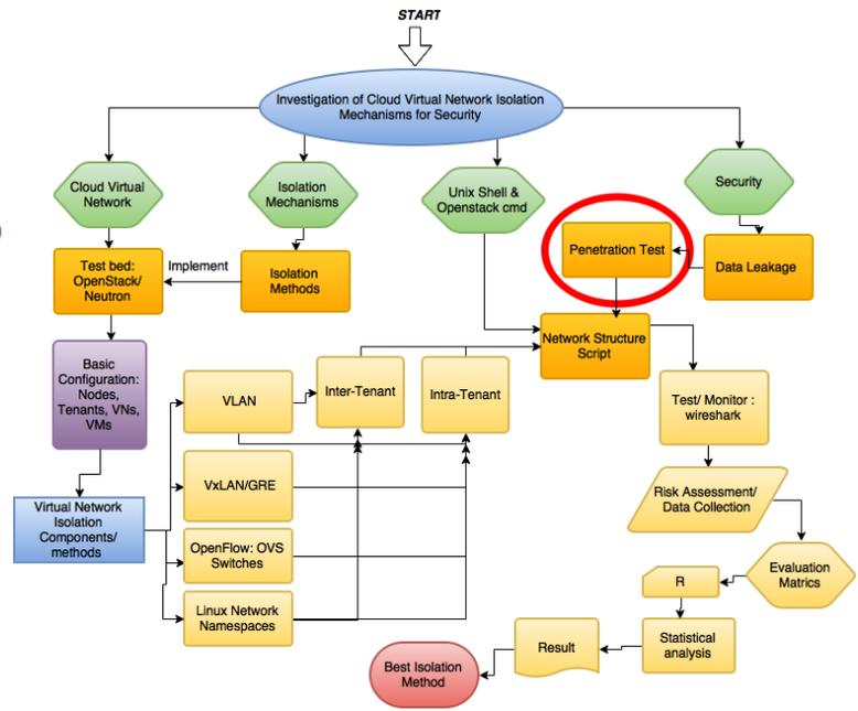
Fig. 2. Test Cloud Virtual Network Isolation with penetration test for data leakage.
