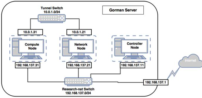
Fig. 1. Three-Nodes OpenStack Cloud Architecture.
